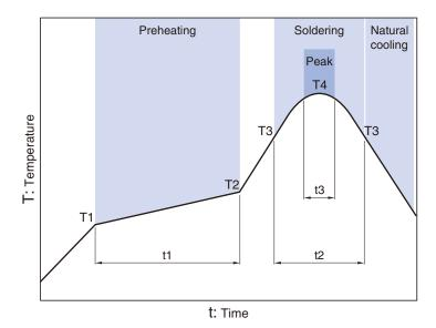
Soldering Preheating Peak Temp. Temp. Temp. Time Time Time T1 T2 T4 Т3 t3 150°C 180°C 60 to 120s 230°C 250 to 260°C 30 to 60s 10s max.
