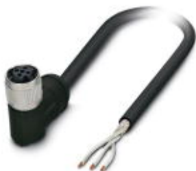
Sensor/actuator cable, 3-position, PE-X halogen-free, black, shielded, free cable end, on Socket angled M12 SPEEDCON, A-coded, cable length: 10 m, For railway applications
