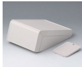
B4056237 UNITEC M, 0.02/0.06 ABS (UL 94 HB) off-white RAL 9002 5.83"x8.27"x3.15" IP 40
