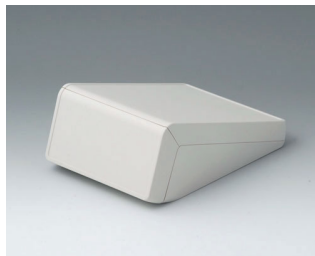
B4054107 UNITEC S, 0.02/0.02 ABS (UL 94 HB) off-white RAL 9002 4.92"x6.97"x2.72" IP 40
