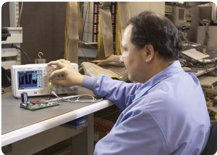
Figure 3. Standard go/no-go mask testing is just one of the reasons manufacturing and service test demand 1000 Series solutions.
