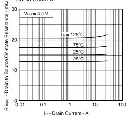
DRAIN TO SOURCE ON-STATE RESISTANCE vs.
