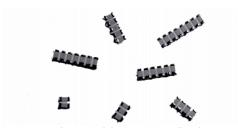
PRA arrays can be used in most applications requiring a matched pair (or set) of resistor elements. The networks provide 1 ppm/°C TCR tracking, a ratio tolerance as tight as 0.01 % and outstanding stability. They are available in 1 mm, 1.35 mm and 1.82 mm pitch.
