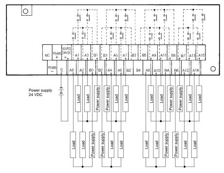
Note: The G730-ROC16/AOM16 is shown above. G730-ROC08 and G730-AOM08 do not have terminals A0 through A7.
