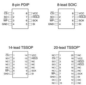
Note: \*Pins 3, 4 and 17, 18 are internally connected for 14-lead TSSOP socket compatibility.
