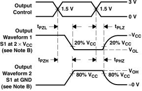
**VOLTAGE WAVEFORMS OUTPUT ENABLE AND DISABLE TIMES**
