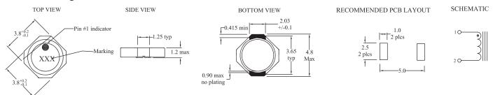
Dimensions are in millimeters.
