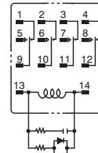
Diagrams show the external dimensions and schematic of the 4 Form C and 4-pole bifurcated (twin) types. For the 1 Form C, 2 Form C, and 3 Form C types, only the terminals differ. The dimensions of the terminal are the same as for standard type HC relays.
