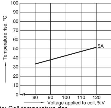
When the nominal voltage is applied to AC 120 or 240 V coil types respectively, the figures of coil temperature rise increase by approx. 10 degrees to the ones shown on each graph.
