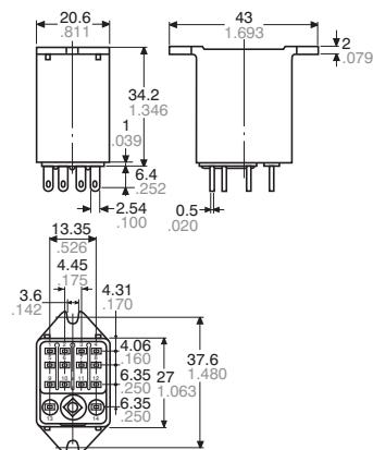
The diagrams show the external dimensions of the 4 Form C and 4-pole bifurcated (twin) types. For 1 Form C, 2 Form C, and 3 Form C, see diagrams at plug-in types (only the terminals are different).
