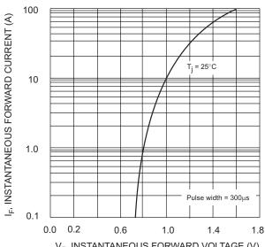
V<sub>F</sub>, INSTANTANEOUS FORWARD VOLTAGE (V) Fig. 2 Typical Forward Characteristics, per element
