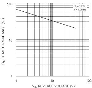
Fig. 4 Typical Total Capacitance, per element
