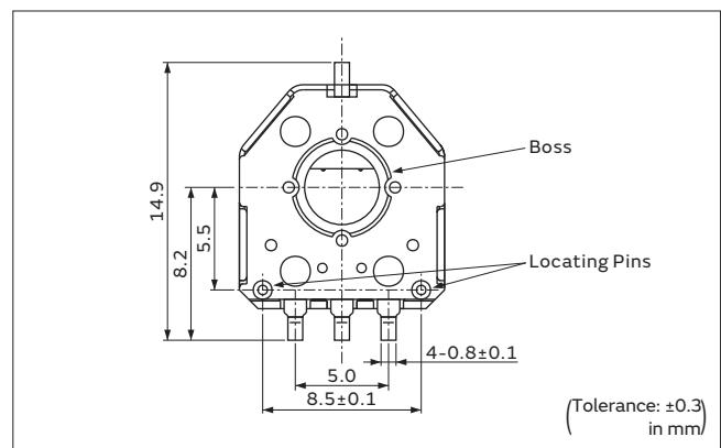
Determine the dimension of the locating holes as follows, depending upon the method of mounting the product (when mounting the product using a mounter or mounting it by hand).
