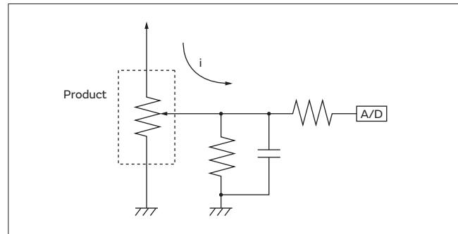
Do not rheostat connect as shown in the figure at right because the contact resistance is slightly high.
