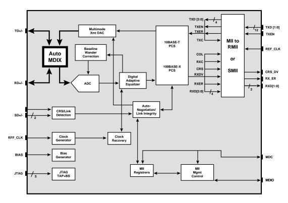
The Broadcom® **BCM5226** is a single-chip device containing six independent Fast Ethernet transceivers. Each performs all the physical layer interface functions for 100BASE-TX full-duplex or half-duplex Ethernet on Category 5 twisted-pair cable and 10BASE-T full or half-duplex Ethernet on Category 3, 4 or 5 cable. Each port may also be configured for 100BASE-FX full or half-duplex transmission over fiber-optic cabling when paired with an external fiber-optic line transceiver.
