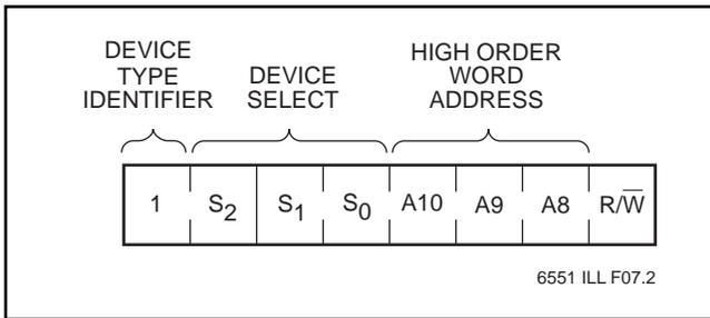
The next three bits of the slave address are an extension of the array's address and are concatenated with the eight bits of address in the word address field, providing direct access to the whole 2048 x 8 array.
