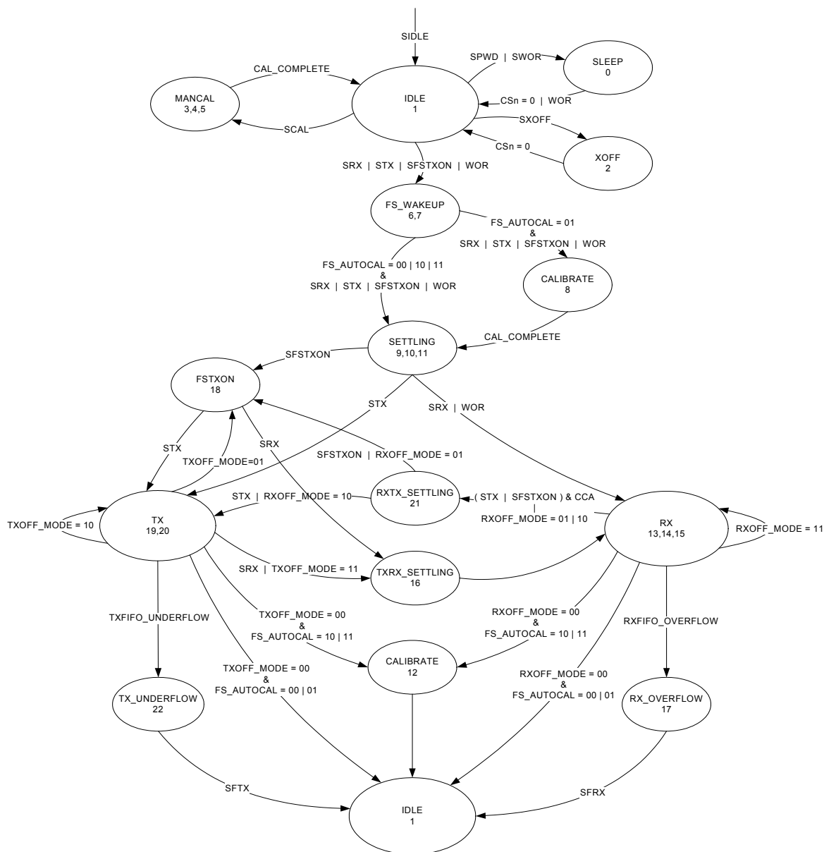
Figure 16: Complete Radio Control State Diagram
