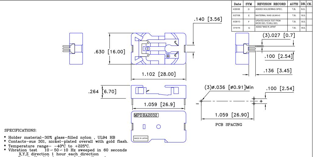
Result: No dislodgement of the cell or damage No discontinuity over 10 micro-seconds.
