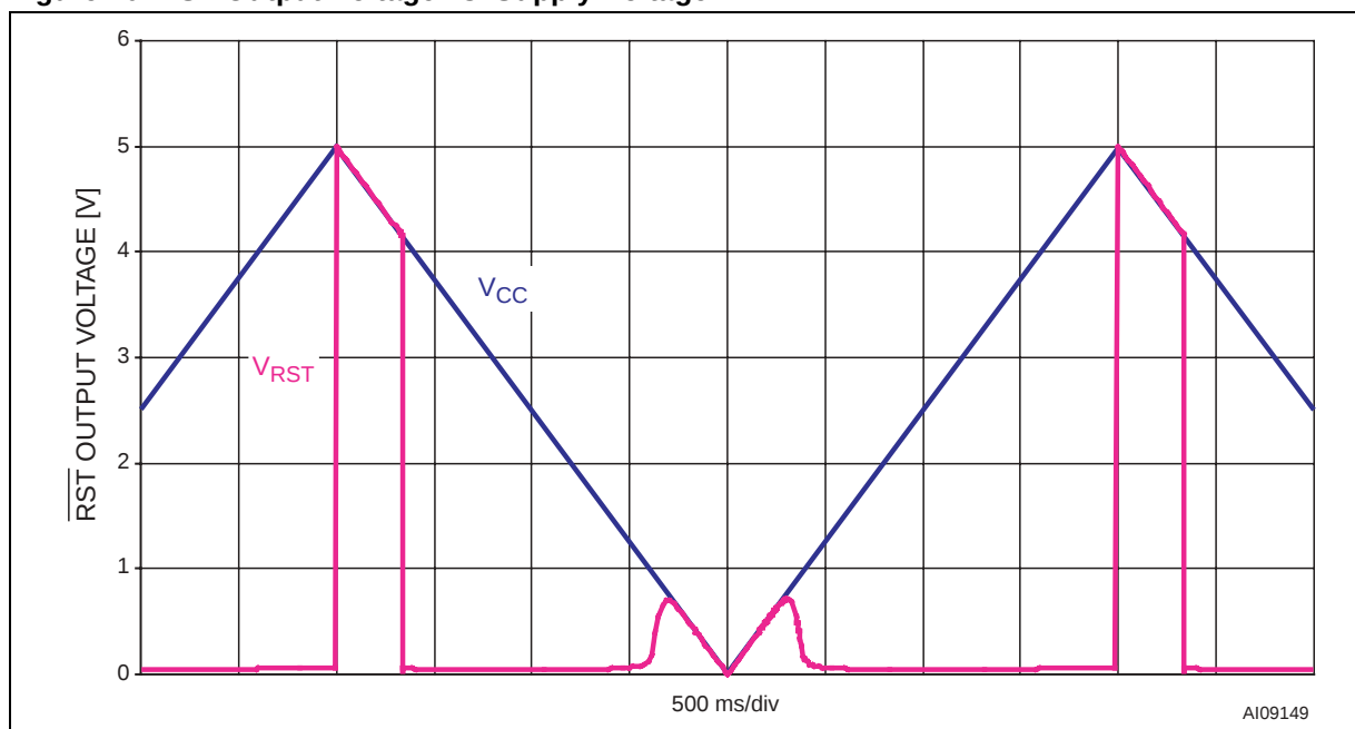
Figure 20. \overline{\text{RST}} Output Voltage vs. Supply Voltage
