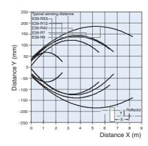
Retro-reflective Models (radial) E3F2-R2R□41-□ (polarizing) and reflectors
