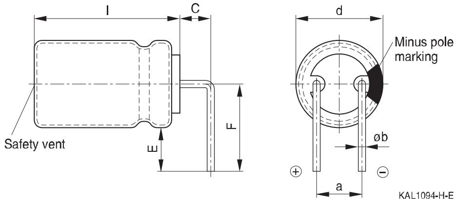
The series B41897 and B41898 have no sleeve nor minus pole marking, the positive pole is marked on the aluminum case side instead.
