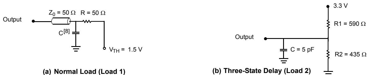
Figure 3. AC Test Load and Waveforms
