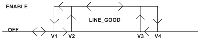
Figure 2. Line UVLO and OVLO Operation
