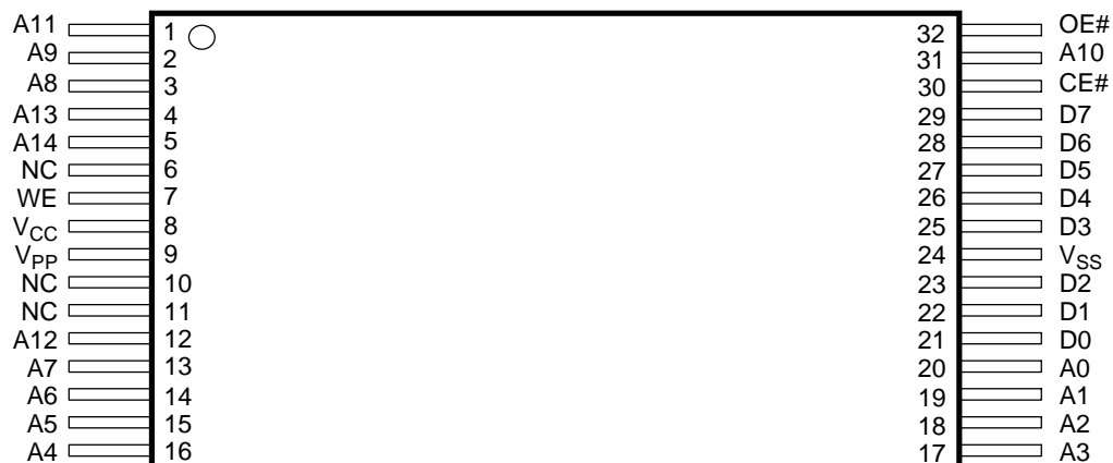
32-Pin — Standard Pinout
