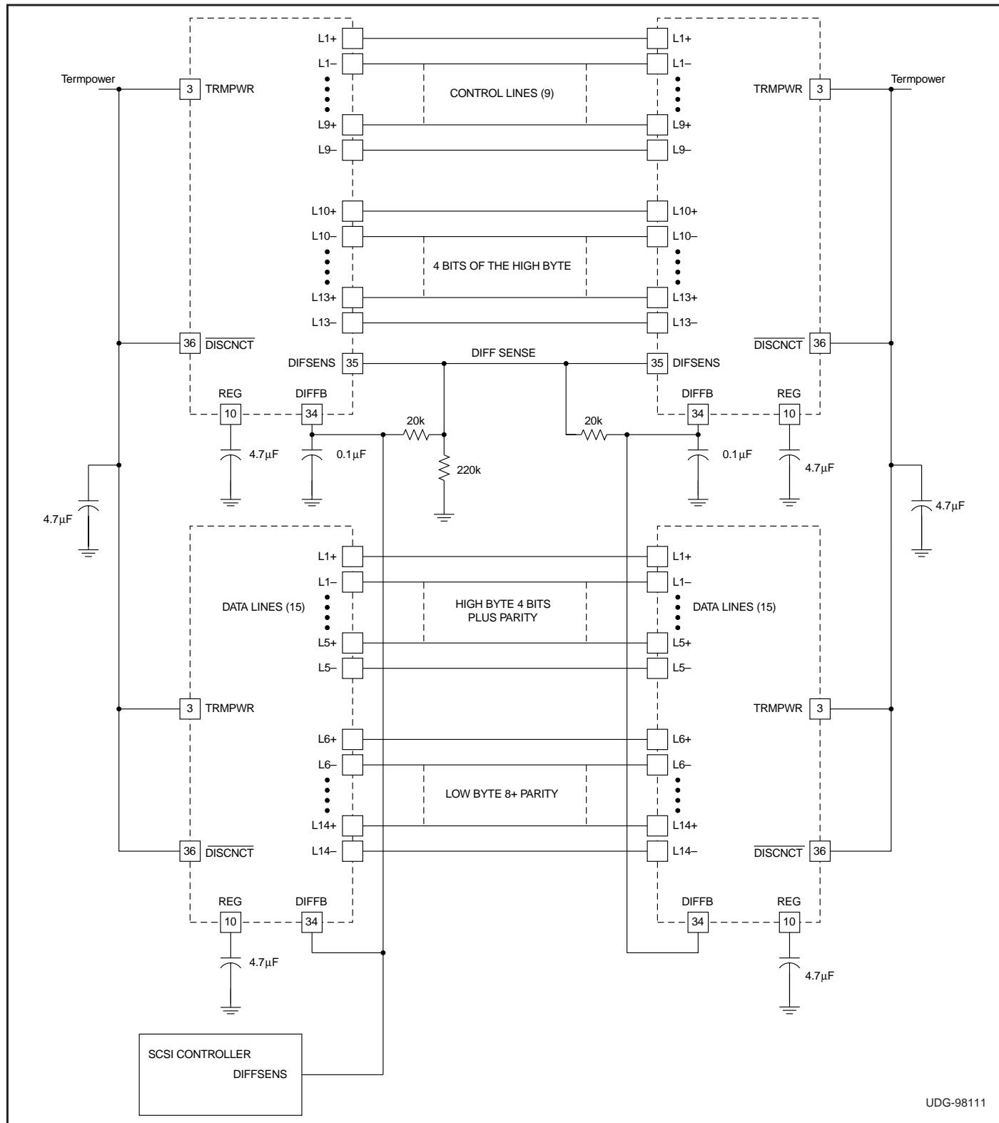
**Note:** A 220k resistor is added to ground to insure the transceivers will come up in single-ended mode when no terminator is enabled. The controller DIFFSENS ties to the DIFFB pin on the terminators, only one RC network should be on a device.
