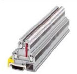
Component terminal block, Connection type: Screw connection, Cross section: 0.2 mm² - 4 mm², AWG: 24 - 10, Nominal current: 34 A, Nominal voltage: 500 V, Length: 66.5 mm, Width: 6.2 mm, Color: gray, Assembly: NS 35/7,5, NS 35/15
