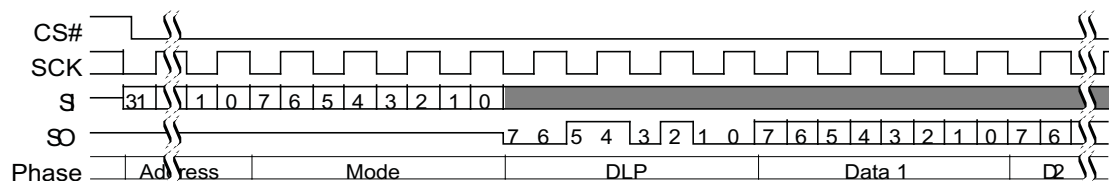
Figure 10.42 Continuous DDR Fast Read Subsequent Access (4-Byte Address [ExtAdd=1, EHPLC=01b])
