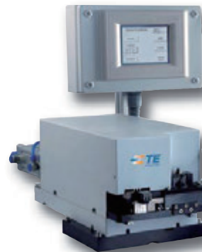
Mark II Inserter with PLC and Insertion Force Control
