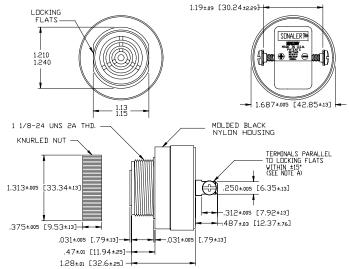
NOTE A: TERMINALS-032 BRASS TIN PLATED, TAPPED FOR #6-32 SCREW. TWO #6-32 NICKEL PLATED BRASS SCREWS INCLUED. WILL ACCEPT 1/4\* QUICK CONNECT. NOTE B: MOUNTING- REMOVE BLACK PLASTIC NUT AND INSERT THREADED FRONT THROUGH L25' HOLE PUNCHED IN PANEL, IF DRIENTATION IS NEEDED, NOTE LOCKING FLATS ON DRAWING. SCREW NUT BACK ON. DO NOT OVERTIGHTEN.
