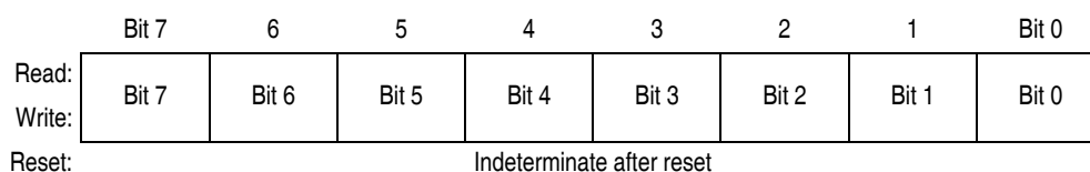
Figure 14-13. TIM Channel Register Low (TCHxL)
