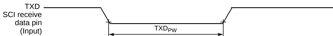
Figure 10-16 TXD Pulse Width
