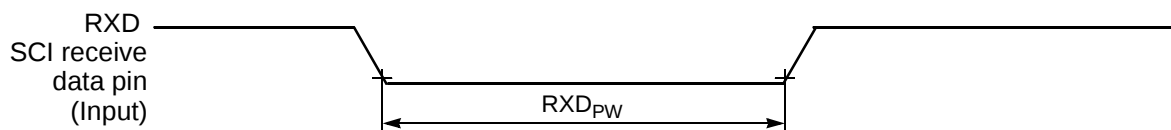
Figure 10-15 RXD Pulse Width
