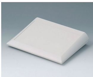
A0620007 COMTEC 200 F, Vers. I ABS (UL 94 HB) off-white RAL 9002 7.87"x5.91"x1.69" IP 40
