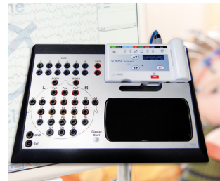
Stationary system for long-term EEG recordings
