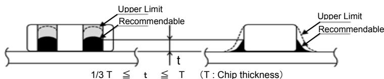
Accordingly increasing the solder volume, the mechanical stress to product is also increased.
