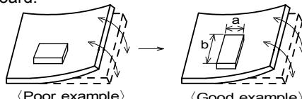
Products shall be located sideways Direction (Length : a<b) to the mechanical Stress.
