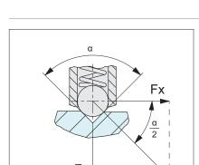
We are able to provide the following formula as an approximation of the pull or push force (N) required to 'release' a ball plunger from its indexing counterpart.
