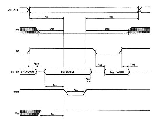
Note: 1. VCC must be applied simultaneously or before Vpp and cut off simultaneously or after Vpp.
