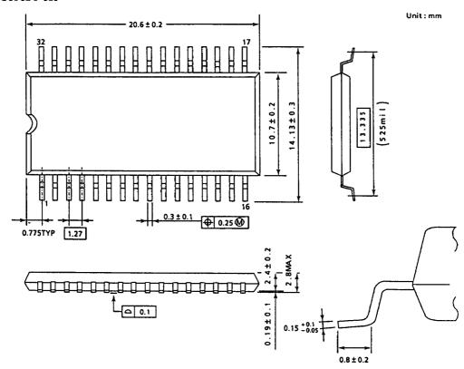
Note: Packge width and length do not include mold protrusion, allowable mold protrusion is 0.15mm
