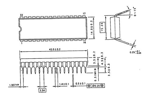
Note: Packge width and length do not include mold protrusion, allowable mold protrusion is 0.15mm
