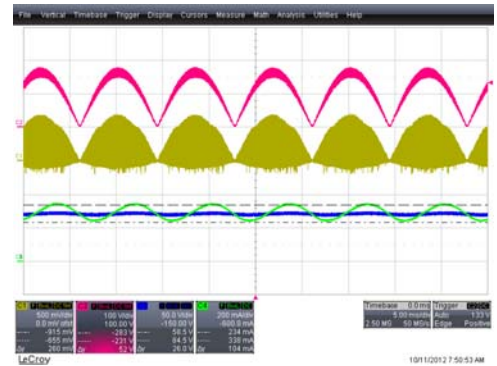
Figure 12. V_{IN} = 120 V_{AC} / 60 \text{ Hz} Operation Waveforms at LED (70 V / 300 mA); C1 [V CS ], C2 [V IN ], C3 [V OUT ], C4 [I OUT ]
