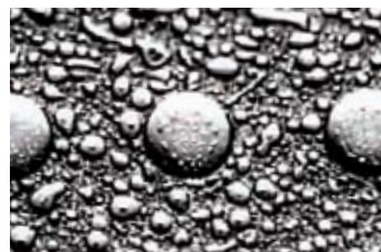
MT Connector Cleaned with IPA
