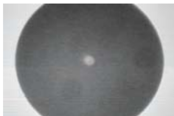
Ceramic Connector Cleaned with Novec Contact Cleaner
