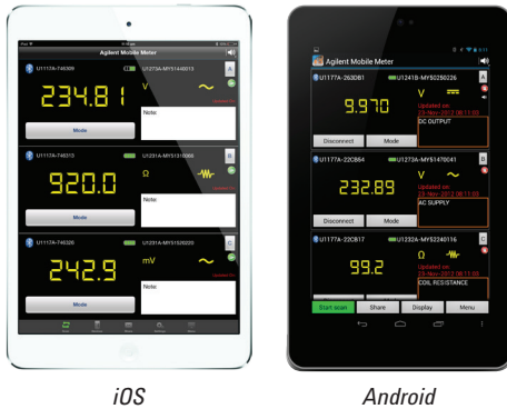
Figure 10. Up to three handheld meters measurements with the Agilent Mobile Meter Application
