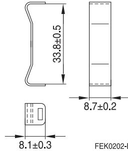
**Coil former (magnetic axis vertical)**
