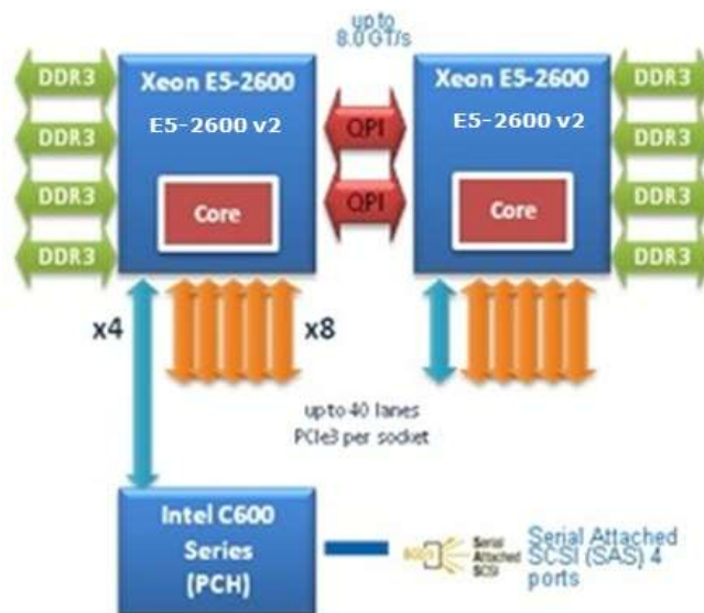
Figure 11. General Functional Block Diagram of Processor I/O Subsystem
