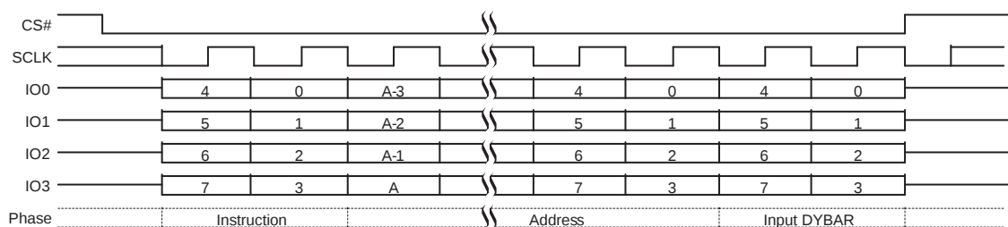
Figure 10.63 DYBWR QPI Mode Command Sequence
