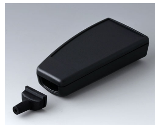
A9066349 SMART-CASE M, Vers. V ABS (UL 94 HB) black RAL 9005 3.78"x1.85"x0.94" IP 40
