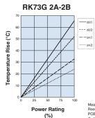
Regarding the temperature rise, the value of the temperature varies per conditions and board for use since the temperature is measured under our measuring conditions.
