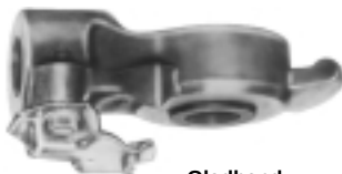
Gladhand Part number 190231-8 1/2-inch female pipe thread
