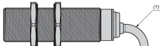
(1) Bending cable: 4 x external cable diameter
