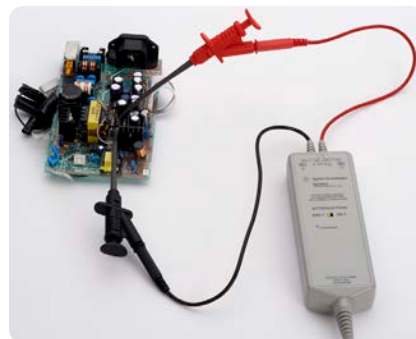
N2790A measuring a power supply signal
