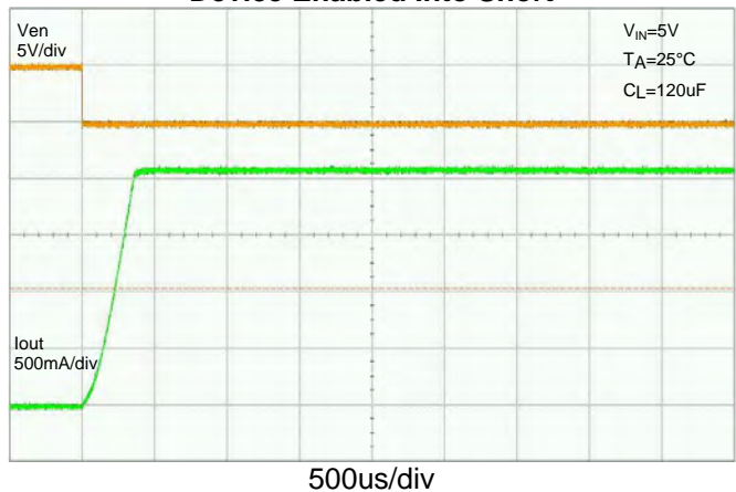
Short Circuit Current, Device Enabled Into Short
