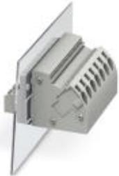
Panel feed-through terminal block, Connection method: Push-in spring connection, Slip-on connection, Load current : 18 A, Cross section: 0.2 mm<sup>2</sup> - 4 mm<sup>2</sup>, AWG 24 - 12, Width: 8.1 mm, Color: gray
