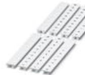
Zack marker strip, can be ordered: Strip, white, labeled according to customer specifications, Mounting type: Snap into tall marker groove, for terminal block width: 8.2 mm, Lettering field: 10.5 x 8.15 mm
