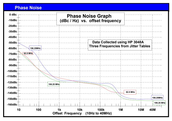
Jitter is frequency dependent. Below are typical values at select frequencies.
