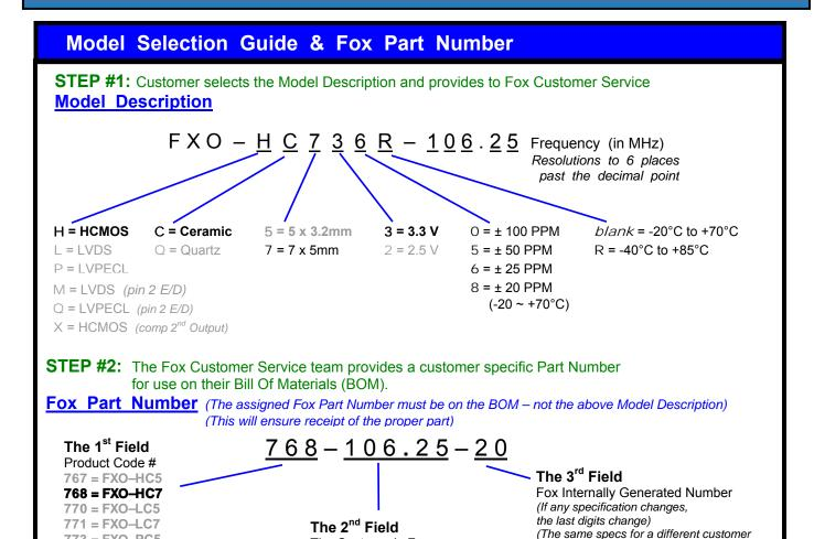
This example, FXO-HC736R-106.25 = HCMOS Output, Ceramic 7 x 5mm Package, 3.3V, ±25 PPM Stability, -40 to +85°C Temperature Range, at 106.25 MHz
