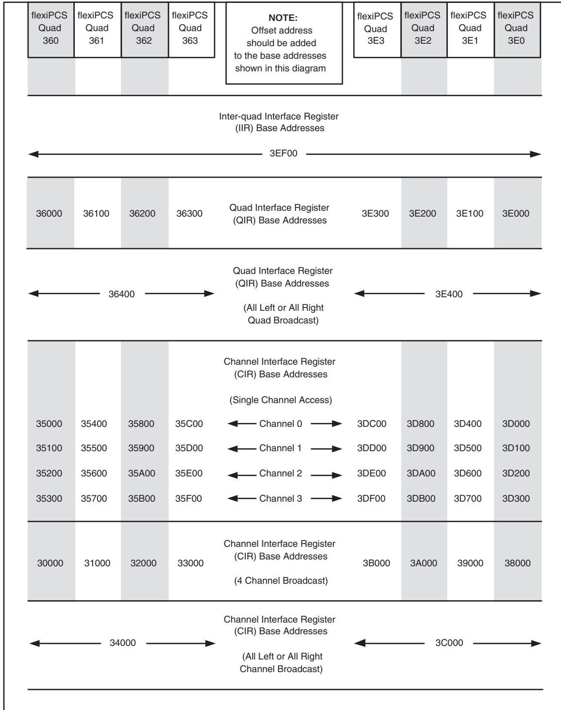
Figure 10-1. flexiPCS Inter-quad, Quad, and Channel Interface Register Map Base Addressing
