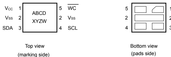
Figure 3. UDFPN5 (DFN5) package connections
